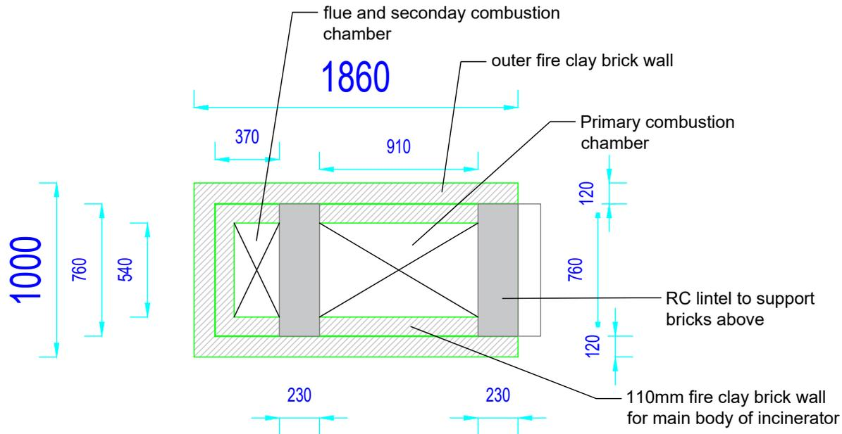
Incinerator floor plan at level 2
